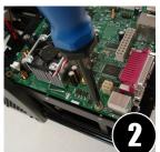
Slide out the Component Tray from the Frame as detailed in section 2.1.
